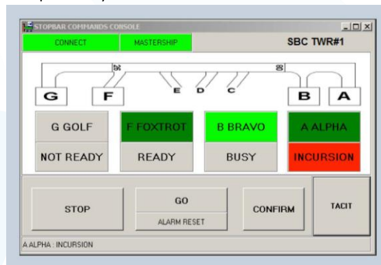
Typical Stop bar Touchpad
